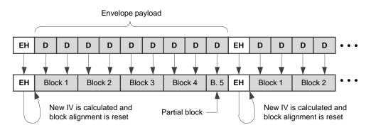
b) Block alignment in an envelope with the payload of odd length
